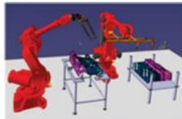
(a) Spot welding configuration with 2 robots and fixtures
